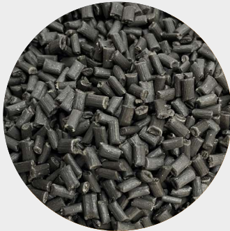
Generated Plastic Beads (PP&PE mixed recycled plastic pellets)
